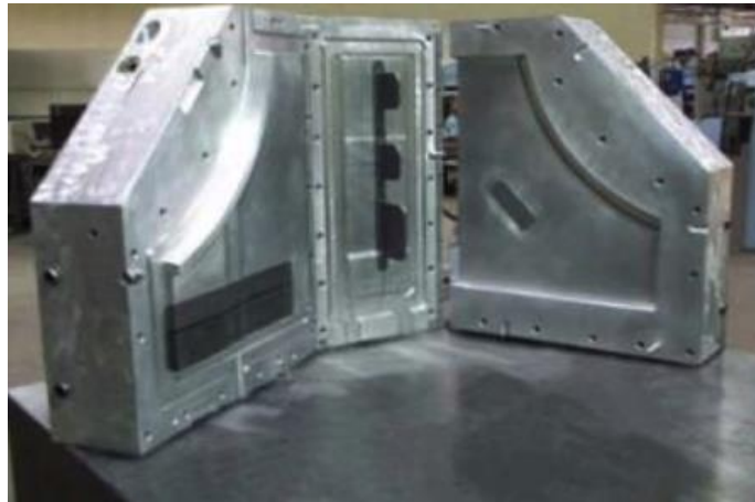
Figure 17 - Molds where the flat mat or preform is put in the RTM manufacturing process.
