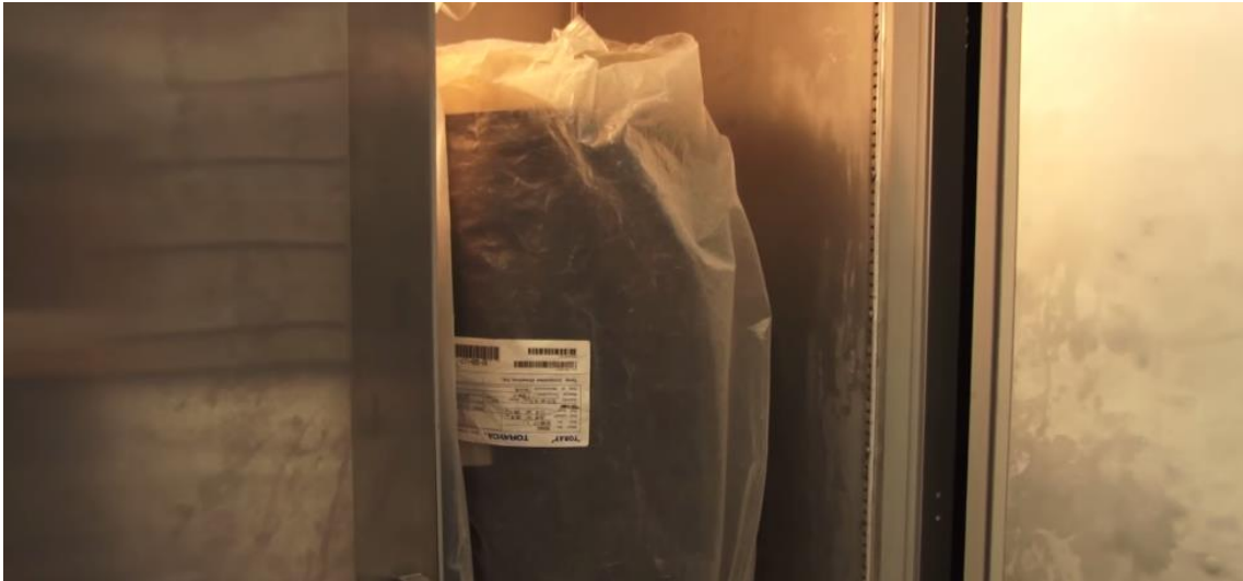
Figure 7 - Removing the prepreg from the freezer. After this let it sit for about 2-3h at room temp.
