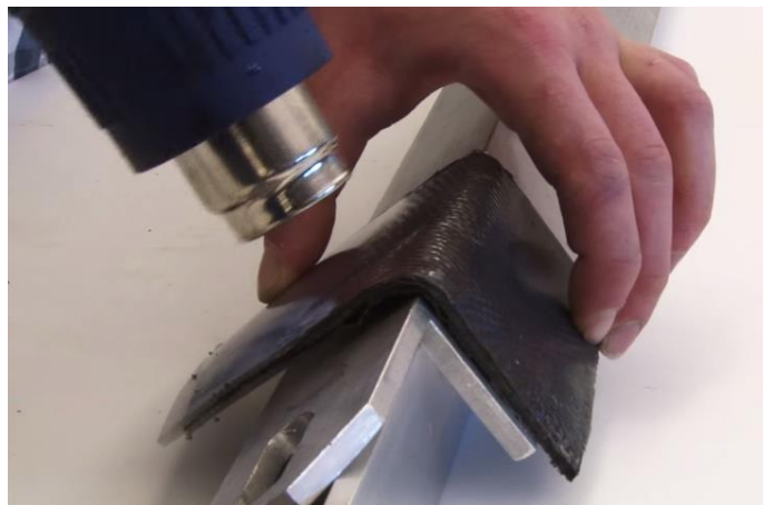
Figure 28 - Heating a composite with thermoplastic matrix to shape it.
