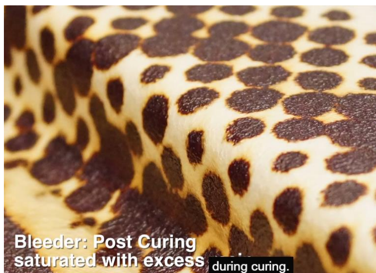
Figure 14 - Bleeder cloth, typically dry glass fibers, to absorb excess epoxy flowing out
