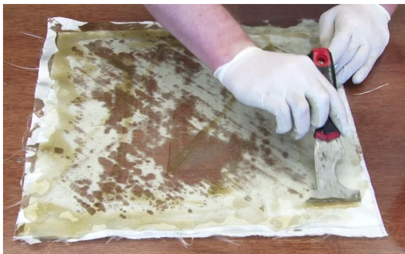
Figure 21 – Applying resin to the fiber cloth.
