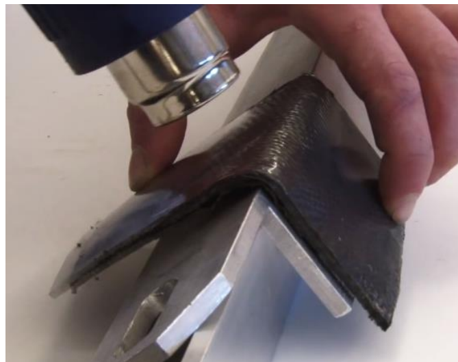
Figure 2 – A thermoplastic composite being heated and molded to a new shape.
