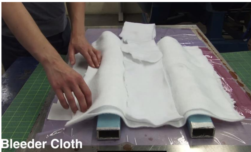
Figure 14 - Bleeder cloth, typically dry glass fibers, to absorb excess epoxy flowing out
