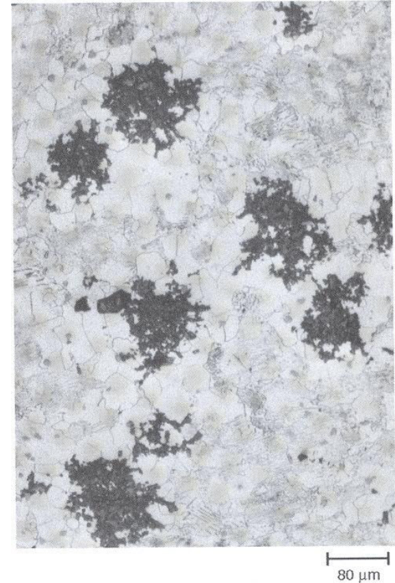
Fig. 92 Malleable iron (Fe-2.95%C-1.2%Si-0.53%Mn-0.06%P-0.21%S-0.08%Cr-0.10%Cu-0.07%Ni-<0.01%Al). The casting was annealed: at 950 °C (1740 °F), held 10 h, furnace cooled to 720 °C (1330 °F), held 16 h, and air cooled. Pearlitic-ferritic matrix. Etched with 4% nital. 125× (microscopic magnification 100×)
