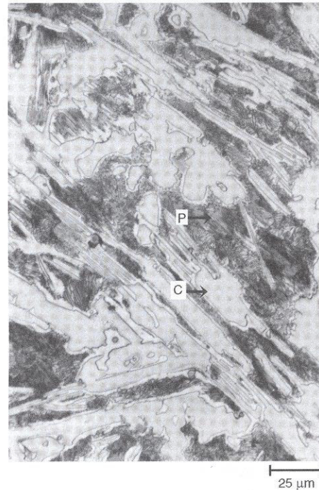
Fig. 94 As-cast white iron (Fe-3.0%C-2.7%Si-0.45%Mn-0.07%P-0.025%S). C, cementite; P, pearlite. Etched with 4% nital. 400×
