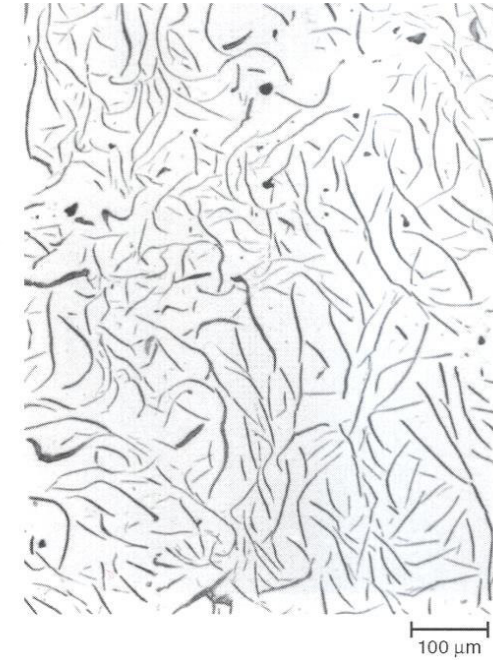
Fig. 60 Hypereutectic as-cast gray iron (Fe-3.5%C-2.95%Si-0.4%Mn-0.08%P-0.02%S-0.13%Ni-0.15%Cu). Flake graphite type A. As-polished. 100×
