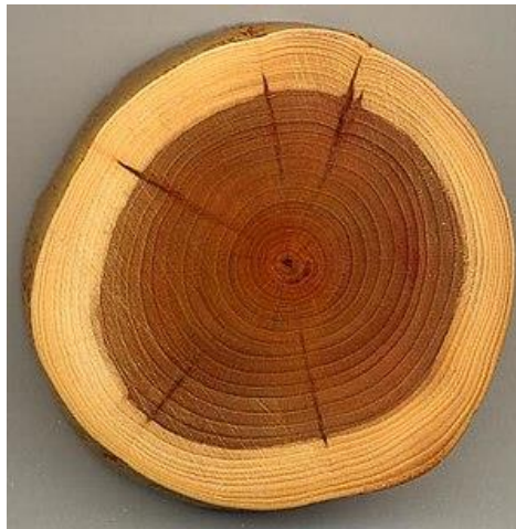
Figure 8 Wood is a specific kind of anisotropic material – orthotropic.
