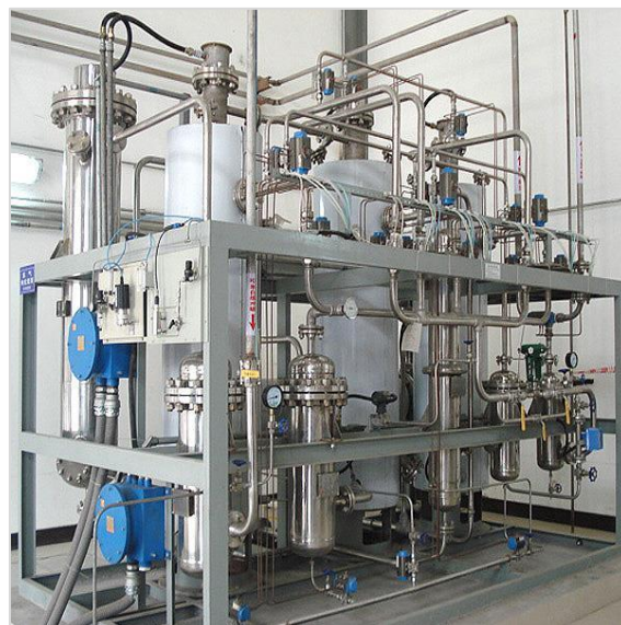
Fig. 11 Example of what a hydrogen purification unit looks like (1).
