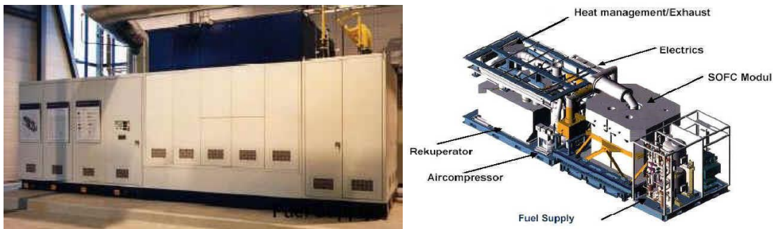
Fig. 48 Siemens Westinghouse 100 kW SOFC (Left) and its main modules (Right) (1).
