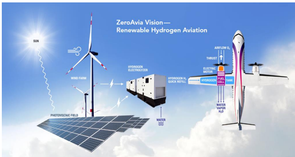
Fig. 30 ZeroAvia's zero emission hydrogen powered airplane for short-haul flights (2).
